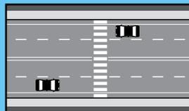
*These marked crosswalks are located in the middle of a block, not at an intersection.*
